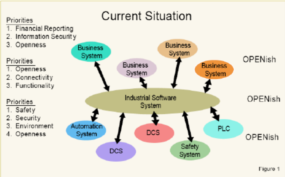
The three traditional classes of automation and information systems, MES, business systems
